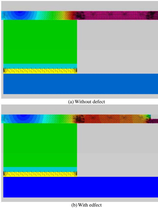
Fig. 2 Distributed magnetization in the pipe by MFL system.
